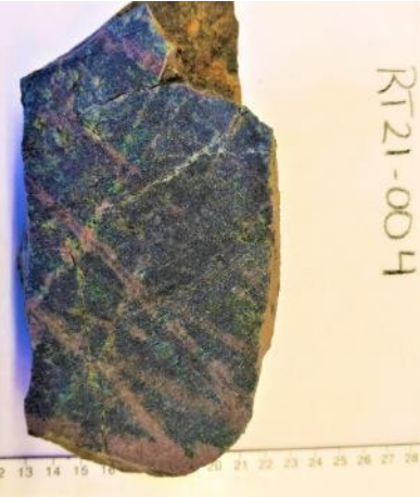
Porphyry-related stockwork pink quartz veins with magnetite and minor chalcopyrite (bornite) in chlorite-magnetite alteration of Jurassic Bonanza Fm. volcanics
